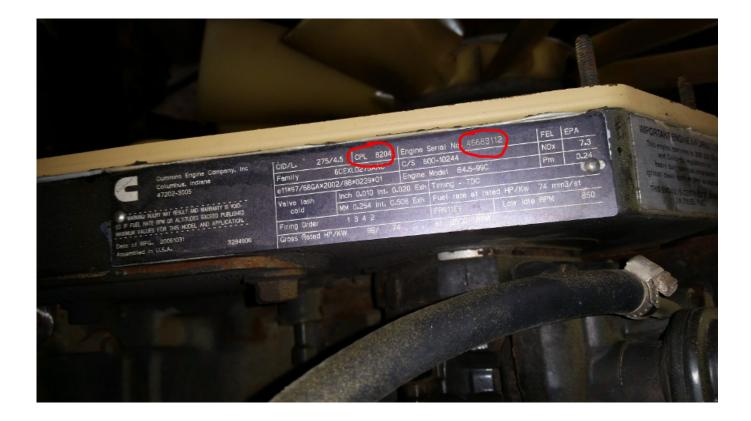
Cummins Engine Serial Number Decoder
